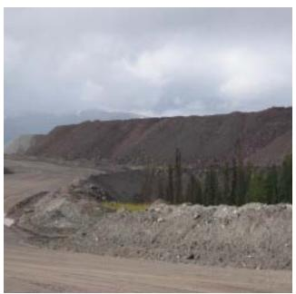
ered if it is to be properly disposed of. The course texture of waste rock allows air and water to easily move through the pile. Because much of the waste rock has never before been exposed to the elements it can be very reactive with the air, water and micro-organisms and may cause *acid mine drainage* (see page 2) and release metals to surface and ground water.
