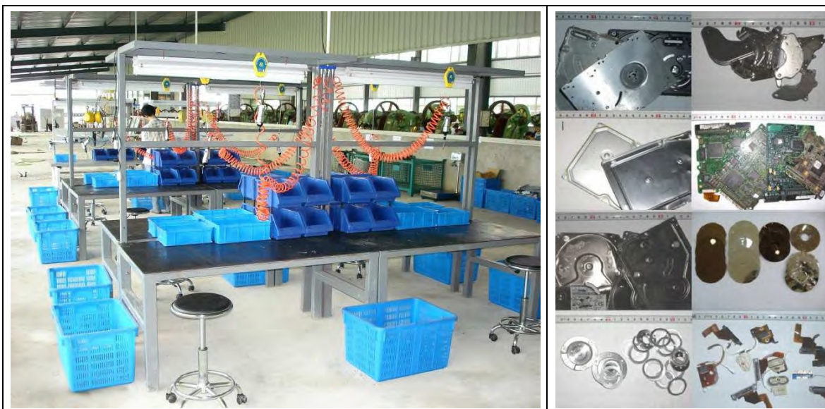
Figure 5-3. Left: Dismantling table with pneumatic tools used for manual dismantling of hard disks. Right: Components resulting from the process and including REE-containing magnets (upper right corner) (Schluep et al., 2009).
