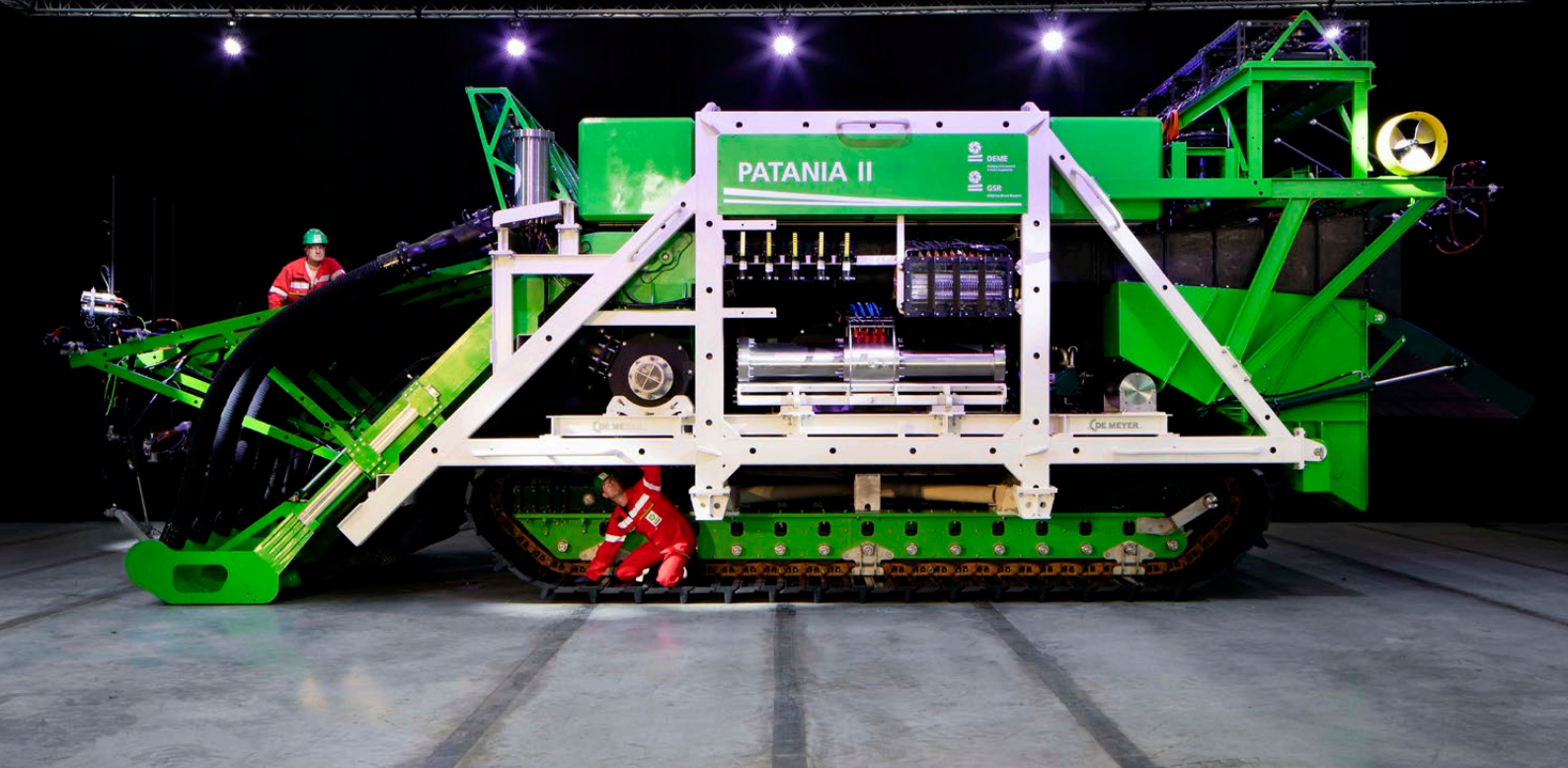
Figure 4 The Patania II which GSR is testing to collect nodules from the seabed in the CCZ Image: DEME Group: https://www2.deme-group.com/
